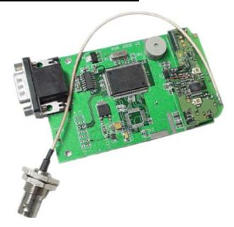
The PSR2000 is a powerful but low cost paging receiver/decoder with a single serial data or TTL output. It incorporates an M16 processor which provides a significant amount of data processing capability.
